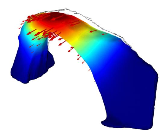
A 3D simulation of resonance mode 1, exaggerated to show the magnitude of displacement. Credit: Jeff Moore
