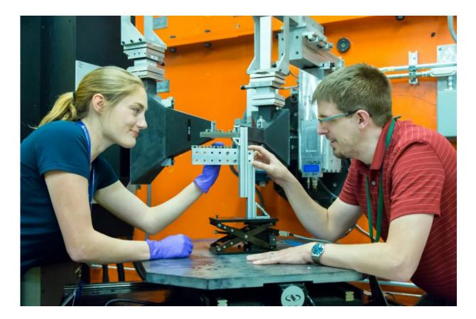
Stacey Bagg, research engineer from NASA's Marshall Space Flight Center, is using HFIR beam line HB-2B, to study residual stress in additive manufactured rocket engine components to qualify them for space flight. Jeff Bunn, right, ORNL postdoctoral research associate and HB-2B instrument team member, assists Bagg with preparing the experiment. Credit: Genevieve Martin/ORNL
