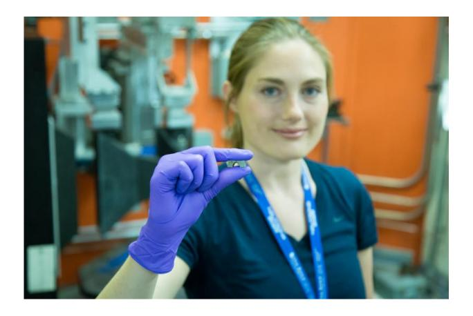
Stacey Bagg, research engineer from NASA's Marshall Space Flight Center, is using HFIR beam line HB-2B, to study residual stress in additive manufactured rocket engine components to qualify them for space flight. Credit: Genevieve Martin/ORNL
