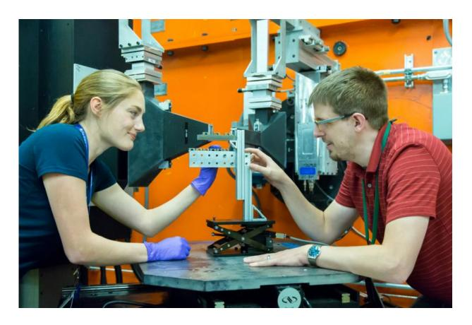
Stacey Bagg, research engineer from NASA's Marshall Space Flight Center, is using HFIR beam line HB-2B, to study residual stress in additive manufactured rocket engine components to qualify them for space flight. Jeff Bunn, right, ORNL postdoctoral research associate and HB-2B instrument team member, assists Bagg with preparing the experiment. Credit: Genevieve Martin/ORNL
