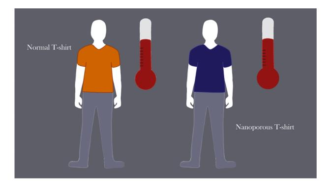
How nanoporous polyethylene reflects visible sunlight, but allow heat to escape. Such material could be used to create clothes that help keep people cool. Credit: Carla Schaffer / AAAS
