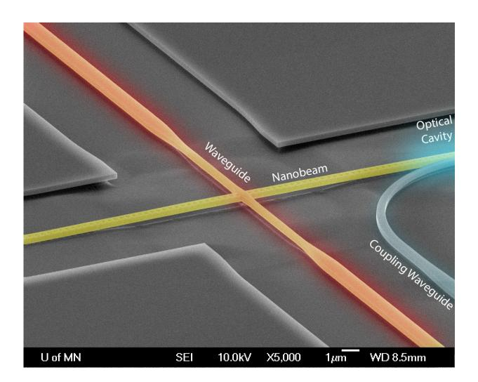
Measurement of the twisting force, or torque, generated by light on a silicon chip holds promise for applications such as miniaturized gyroscopes and sensors to measure magnetic field, which can have significant industrial and consumer impact. Credit: University of Minnesota
