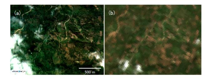
This graphic compares two RGB images of Dumingag on the island of Mindanao, Philippines. Image (a) was taken by the HPT installed in DIWATA-1, while image (b) was taken by Landsat 8's OLI. These results demonstrate that DIWATA-1 can observe the Earth at significantly higher resolutions than existing large satellites. Credit: Hokkaido University
