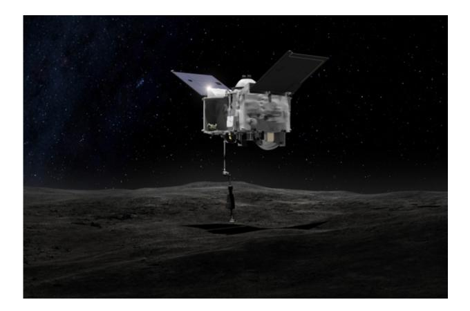
This artist's depiction shows the OSIRIS-REx spacecraft contacting the asteroid Bennu with its Touch-And-Go Sample Arm. The mission aims to return a sample of Bennu's surface coating to Earth and to return detailed information about the asteroid and its trajectory. Credit: NASA's Goddard Space Flight Center
