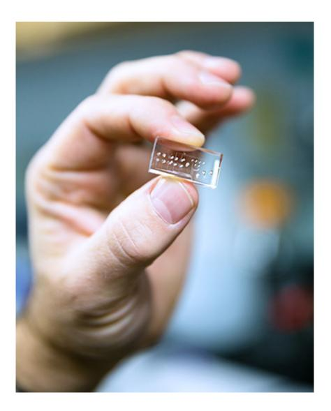
A new optofluidic platform for biological sample processing and optical analysis is made of polydimethylsiloxane (PDMS) and features tunable optics and novel 'lightvalves.' . Credit: C. Lagattuta
