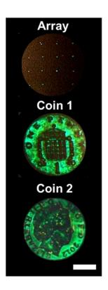
Rewritable holographic array and 3D virtual images of coins. Scale bar: 5mm. Credit: Yetisen et al. ©2016 AIP Publishing
