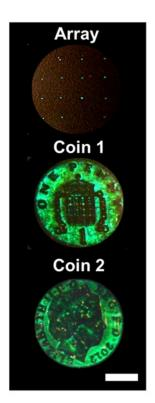
Rewritable holographic array and 3D virtual images of coins. Scale bar: 5mm. Credit: Yetisen et al. ©2016 AIP Publishing
