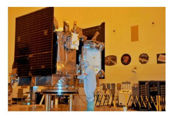
The OSIRIS-REx spacecraft sits on its workstand while an engineer checks the protective covering in a servicing building at Kennedy Space Center, Florida
