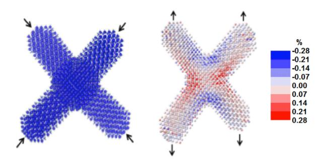
These atom-scale computer simulations of tetrapods show how they sense compression (left) and tension along one axis (right), both of which are crucial to detecting nanoscale crack formation. The color bar indicates the percent change of the tetrapods' volume. Credit: Berkeley Lab
