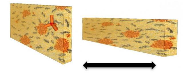
This schematic shows a tetrapod-polymer film before and after it is stretched length-wise. The orange areas are clusters of tetrapods. The scientists found the color of light emitted by the tetrapods changed when the polymer was stretched. Credit: Berkeley Lab
