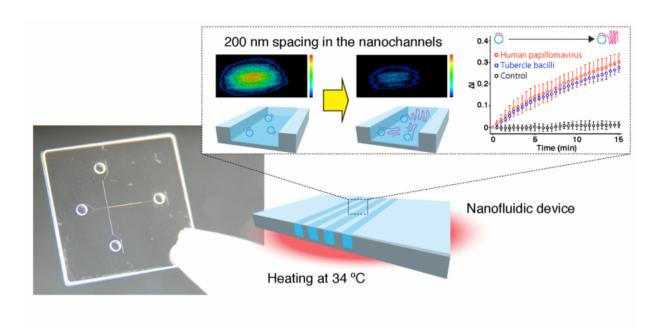
A photo and a schematic illustration for a nanofluidic diffraction grating. Labelfree signals based on a diffraction intensity change were attributed to amplification of DNA molecules, such as human papillomavirus and tubercle bacilli. Credit: Takao Yasui
