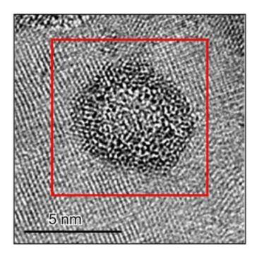
BF-STEM image highlighting the core–shell structure of the nanocluster. Credit: *Nature* (2016). DOI: 10.1038/nature19313
