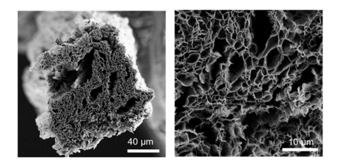
Scanning electron microscopy imagery of a graphene fiber made from microwave reduced graphene oxide. Credit: Jieun Yang, Damien Voiry and Jacob Kupferberg
