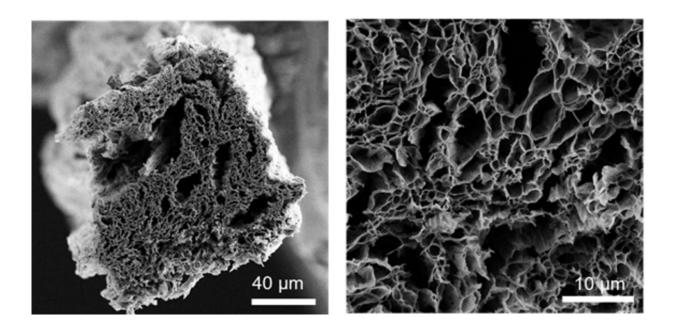
Scanning electron microscopy imagery of a graphene fiber made from microwave reduced graphene oxide. Credit: Jieun Yang, Damien Voiry and Jacob Kupferberg
