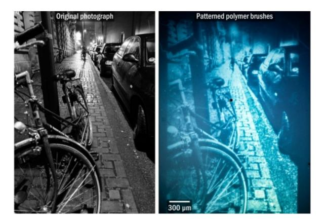
The stop-flow photopatterning method allows for the creation of intricate polymer brush patterns Credit: Christian Pester
