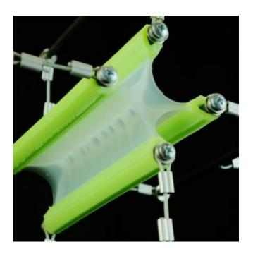
The team's experimental setup stretched a thick, soft elastomer — made from silicon rubber — at each of its corners. Under this biaxial tension, the sample's center deformed, breaking the geometrical symmetry and becoming suddenly flat. Credit: Johannes T.B. Overvelde/Harvard SEAS
