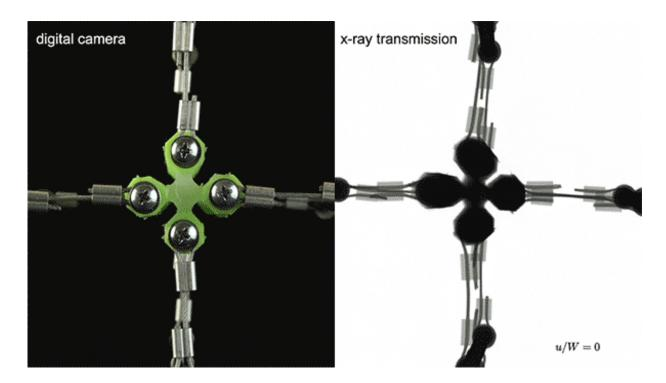
A soft architected material that, due to the tension instability, undergoes a pattern transformation when biaxially stretched. Credit: Johannes T.B. Overvelde/Harvard SEAS
