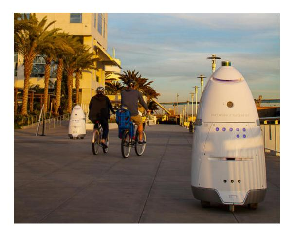
In this April 19, 2016, photo, provided by Stacy Dean Stephens, Knightscope K5 security robots, at right, and background left, patrol alongside a pier, in San Diego. The robots can identify a vehicle parked in a certain location for too long or sense intruders at odd hours. The company expects to have several large mall developers in California start using the robots in late 2016. (Stacy Dean Stephens via AP)
