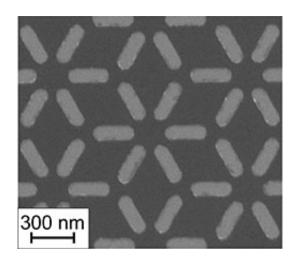
Electron microscopy image of a small fraction of the dipolar dice lattice. The spin ice structure consists of interacting ferromagnetic nanoislands. The experimental lattice consists of several thousand nanoislands and is fabricated by electron-beam lithography. Credit: Aalto University
