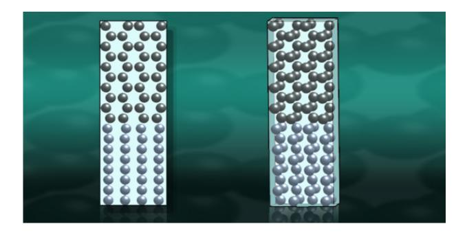
Ten layers of hexagonal iron (dark gray) above eight layers of cubic iron (pale blue-gray). Each layer can transform from one structure to the other by pinching pairs of adjacent atoms toward or away from one another. Lawrence Livermore researchers calculated the structural transformation of iron, showing how it springs back to shape under pressure. Credit: Lawrence Livermore National Laboratory
