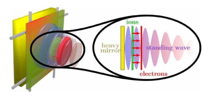
A laser beam (from the right) falls onto a thin foil, with a mirror on the rear side. The beam is reflected, forming a standing wave. Because of the systematical variation in wavelength of the laser pulse, the crests of the wave start to move. This drags the electrons (red) and ions (green) along, accelerating them to high speeds in the direction of the arrows. Credit: Felix Mackenroth
