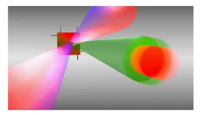
A laser beam (purple-red) falls onto a thin foil, with a mirror on the rear side. The beam is reflected, forming a standing wave. Because of the systematical variation in wavelength of the laser pulse, the crests of the wave start to move. This drags the electrons and ions along, accelerating them to high speeds (green beam). Credit: Felix Mackenroth
