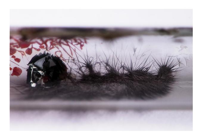
On the left side crystals of residual black phosphorus and tiniodide. The material is easy to produce and shows extraordinary optical and electronic properties, as well as extreme mechanical flexibility. Credit: Andreas Battenberg / TUM
