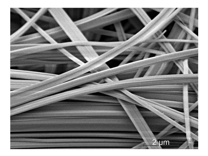
Electron<br/>microscopic image of SnIP-needles (9700x, 5 kV) . Credit: Viola Duppel / MPI for Solid State Research
