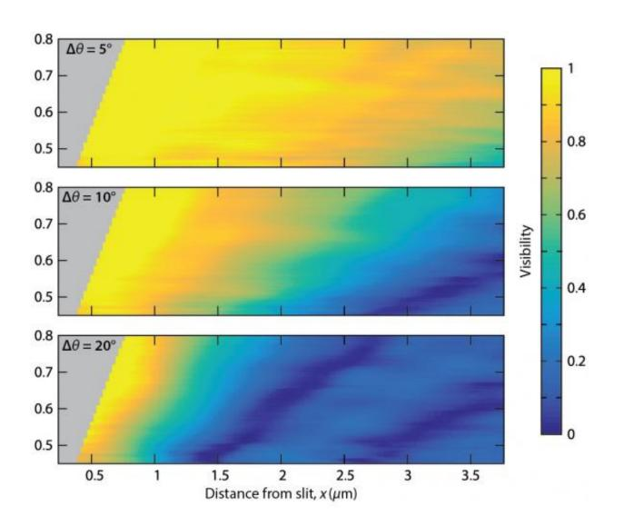
A new technique detects spatial coherence in light at smaller scales than had been possible. The image shows visibility curves appearing at the nanoscale, the telltale sign of spatial coherence. Credit: Pacifici Lab / Brown University
