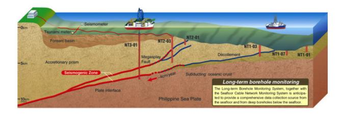
Cross-section of the location where the IODP team installed new monitoring equipment. Credit: The NanTroSEIZE Scientific Team - CC BY-SA 3.0
