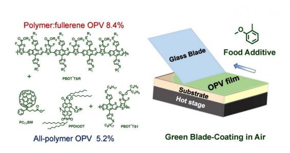
Schematic illustration and chemical structure of semi-printed plastic solar cells in air, using food additive o-MA as solvent. Image credit: Long Ye, NC State
