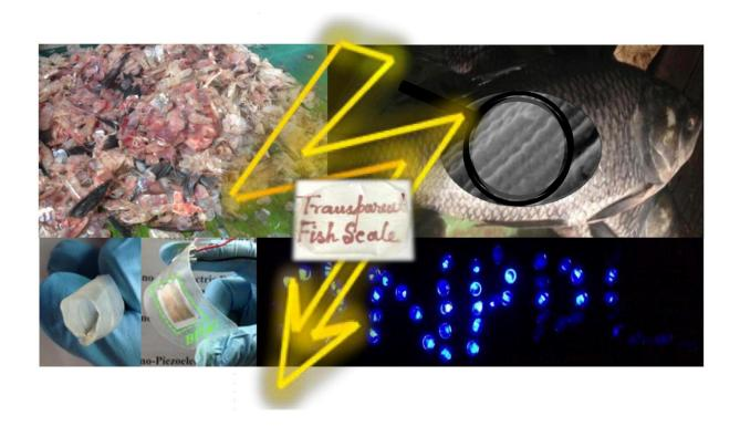
Waste fish scales (upper left corner) are used to fabricate flexible nanogenerator (lower left) that power up more than 50 blue LEDs (lower right). An enlarged microscopic view of a fish scale shows the well-aligned collagen fibrils (upper right). The possibility of making a fish scale transparent (middle) and rollable (extreme left lower corner) is also illustrated. Credit: Sujoy Kuman Ghosh and Dipankar Mandal/Jadavpur University
