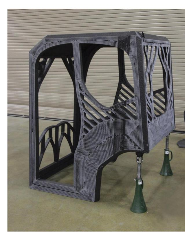
The first-ever 3D printed excavator will include a cab designed by a University of Illinois at Urbana-Champaign student engineering team and printed at DOE's
