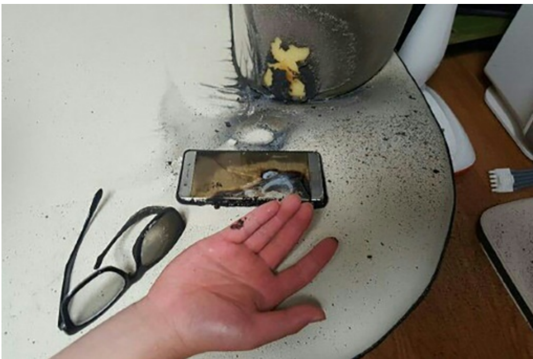
A blown-up Samsung Galaxy Note7 smartphone pictured in Gwangju
