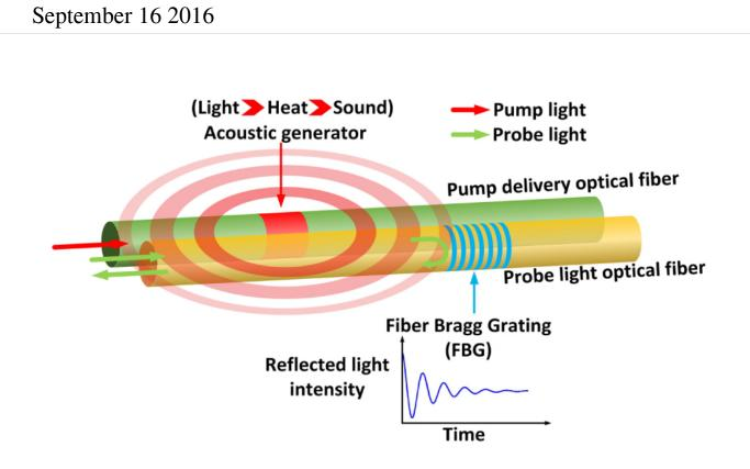
The principle of operation for a single AFO-SHM sensing node. Credit: *Optics Express* (2016). DOI: 10.1364/OE.24.020287
