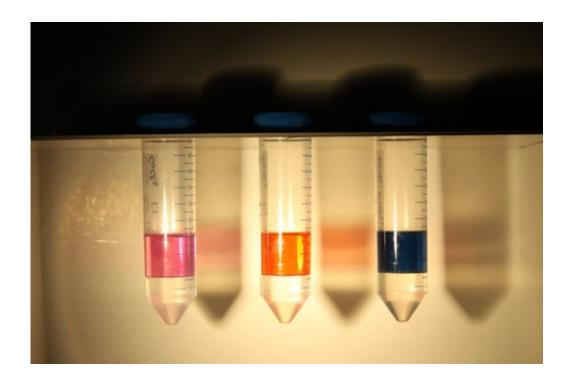
Three tubes with a layer of purified water at the bottom; above a layer of DES containing the metal ions. From left to right, the tubes in which cobalt, iron and a combination of cobalt, copper, nickel and zinc respectively have been removed. Credit: Eindhoven University of Technology
