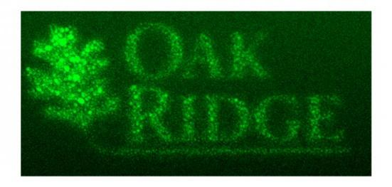
To direct-write the logo of the Department of Energy's Oak Ridge National Laboratory, scientists started with a gray-scale image. They used the electron beam of an aberration-corrected scanning transmission electron microscope to induce palladium from a solution to deposit as nanocrystals. Credit: Oak Ridge National Laboratory, U.S. Dept. of Energy
