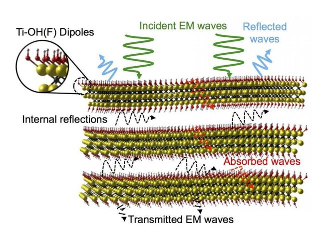
Drexel University researchers have demonstrated that MXene can be a highly effective, light weight, low volume shield to protect electronics devices from electromagnetic interference. Credit: Drexel University
