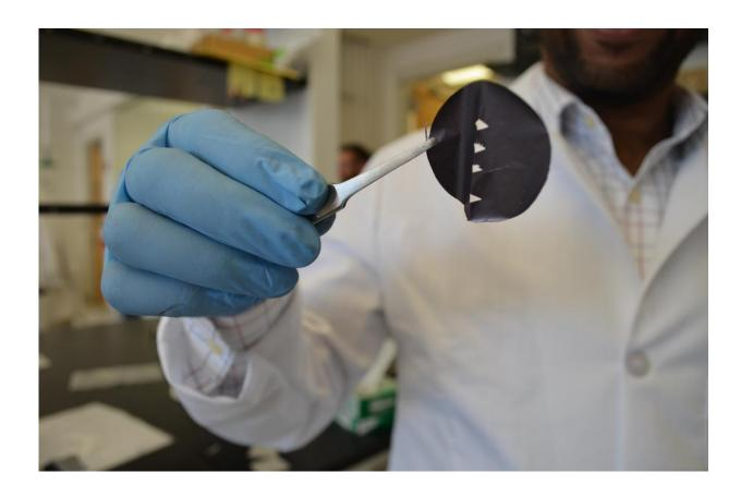
Researchers at Drexel University have developed a nanomaterial, called MXene, that could potentially be used in electronics devices to block out and insulate electromagnetic waves. Credit: Drexel University
