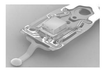
The slider and recording head assembly that writes data to modern hard disk drives. Credit: IOP Publishing
