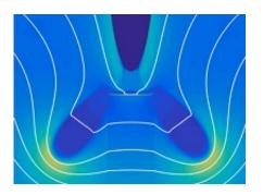
Detail of a simulation of a pulsed positive discharge near a dielectric rod, made by Anna Dubinova. Credit: CWI
