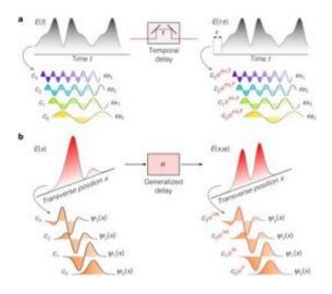
Generalized Optical Interferometry Using a Hilbert-space analyzer. A beam is directed to an interferometer and is split between two paths, the lower of which contains a generalized delay ( $\alpha$ ) replacing the usual temporal delay. Then the two beams are recombined to produce an interferogram. Credit: Ayman F. Abouraddy
