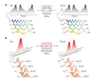
Generalized Optical Interferometry Using a Hilbert-space analyzer. A beam is directed to an interferometer and is split between two paths, the lower of which contains a generalized delay ( $\alpha$ ) replacing the usual temporal delay. Then the two beams are recombined to produce an interferogram. Credit: Ayman F. Abouraddy
