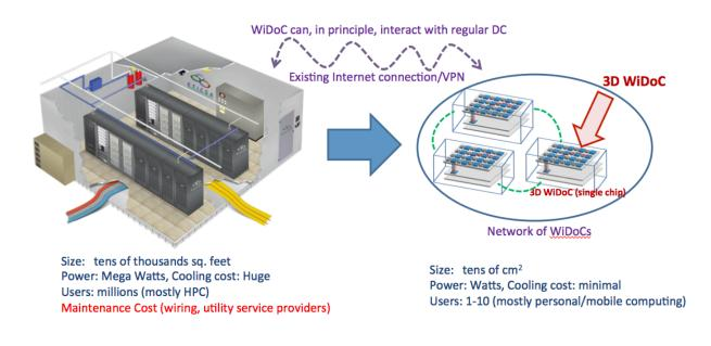
From Data Centers to Wireless Datacenter on Chip (WiDoCs). Credit: Carnegie Mellon University Electrical and Computer Engineering
