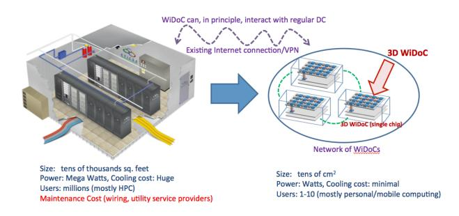
From Data Centers to Wireless Datacenter on Chip (WiDoCs). Credit: Carnegie Mellon University Electrical and Computer Engineering
