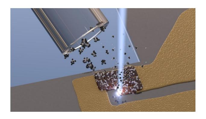
The sensor is made up of highly conductive platinum nanoparticles surrounded by an insulating carbon matrix. Credit: 2016 EPFL
