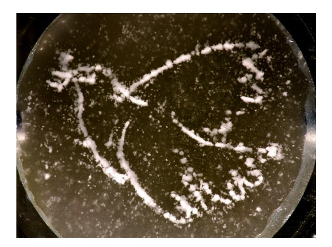
Shaped with ultrasound: Max Planck researchers from Stuttgart transmit ultrasonic waves through a bath of water and microparticles. In doing so, they model the profile of the sound pressure with a hologram in such manner that the particles are pushed into the shape of Picasso's peace dove. Credit: Kai Melde / MPI for Intelligent Systems
