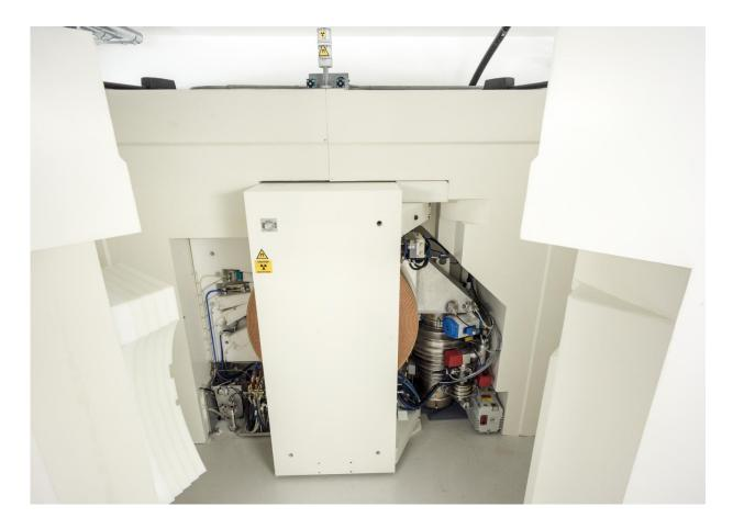
The cyclotron with open radiation shield shows a view on the targets (left), the magnets and the cyclotron itself (center), and the vacuum system (right). Credit: photo/©: Stefan F. Sämmer, JGU
