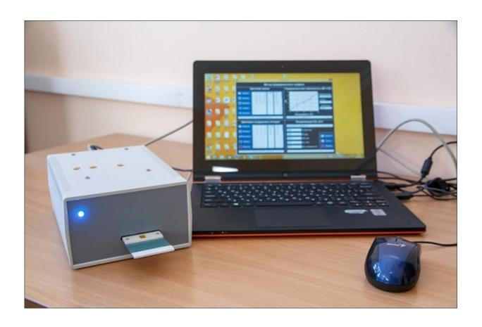
The portable device for water analysis. Credit: Tomsk Polytechnic University (TPU)
