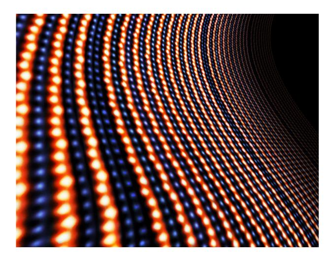
Scientists engineered a new magnetic ferroelectric at the atomic-scale. A false-colored electron microscopy image shows alternating lutetium (yellow) and iron (blue) atomic planes. An extra plane of iron atoms was inserted every ten repeats, substantially changing the magnetic properties. Credit: Emily Ryan and Megan Holtz/Cornell
