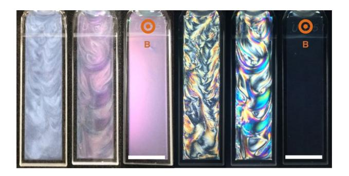
(Left) Three optical images and (right) three polarized optical images of photonic water. Credit: K. Sano et al. ©2016 Nature Communications
