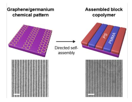
Chemical patterns consisting of alternating graphene and germanium stripes (left side) are used to direct the self-assembly of block copolymers into well-ordered patterns (right side). The top images are schematics and the bottom images are scanning electron micrographs. The scale bars are 200 nm. Credit: University of Wisconsin-Madison
