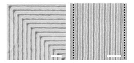
Scanning electron micrographs of block copolymer films assembled on graphene/germanium chemical patterns with 90 degree bends (left side) and with density multiplication by a factor of 10 (right side). The black dotted lines (right side) indicate the period of the graphene/germanium chemical pattern, in which the period of the assembled block copolymer is reduced by a factor of 10 due to density multiplication. The scale bars are 200 nm. Credit: University of Wisconsin-Madison
