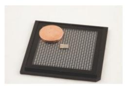
Using photonic integrated circuit technology, researchers made a tiny, yet fast quantum random number generator. The small chip in the middle of the picture contains two of the random number generators, which together measure 6 by 2 millimeters. For comparison, the coin is 16.25 millimeters in diameter. Credit: Daniel Bartolome & Ona Bombí, ICFO
