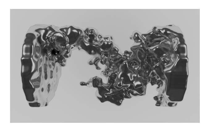
NYU chemists and their colleagues have developed a method to yield highly detailed, three-dimensional images of the insides of batteries. Shown here is a 3-D image of the inside of a lithium cell after charging and showing dendrite growth -- deposits than can reduce performance and compromise safety -- between the two electrodes that short-circuited the cell. Credit: NYU's Jerschow lab
