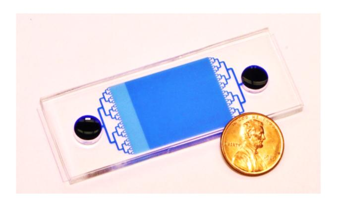
The channel through the chip splits into 64 branches, each with 200 chambers along it for trapping single cells. Credit: Yoon Lab, University of Michigan
