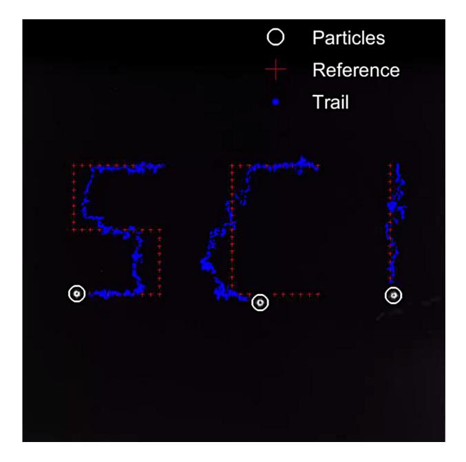
Researchers move multiple objects simultaneously on a metal plate by playing a carefully chosen melody. Credit: Quan Zhou / Aalto University
