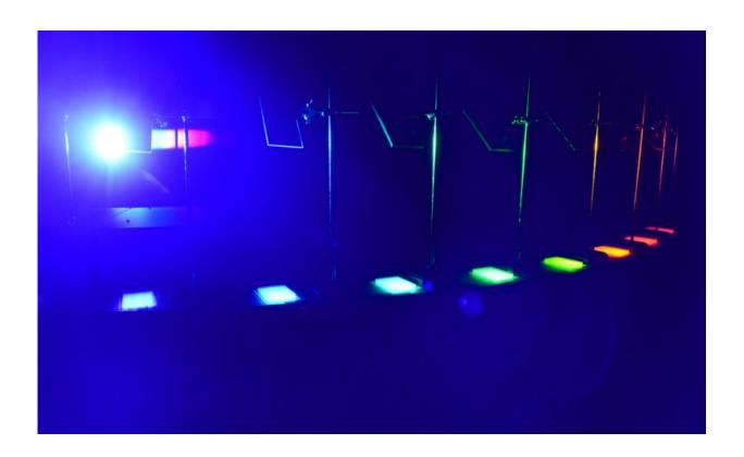
Okazaki Large Spectrograph in Japan, where the action spectra of qE quenching were recorded. Credit: NIBB
