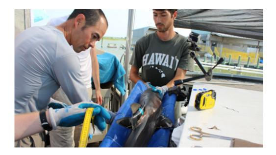
The accelerometer (made waterproof inside heat-shrink tubing) attaches to the shark's dorsal fin. Credit: Marisa Spyker
