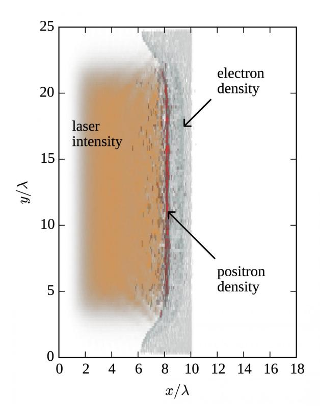
The distribution of the laser intensity (orange), the foil electron and foil ion densities (gray), and the positron density (red) in the x-y plane. The laser pulse
