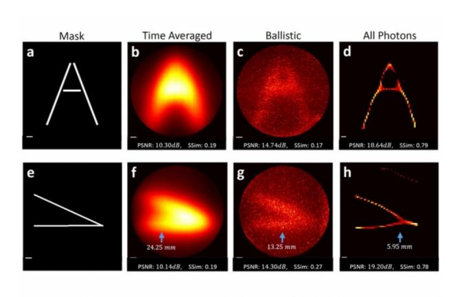
In experiments, the researchers fired a laser beam through a "mask" — a thick sheet of plastic with slits cut through it in a certain configuration, such as the letter A — and then through a 1.5-centimeter "tissue phantom," a slab of material designed to mimic the optical properties of human tissue for purposes of calibrating imaging systems. Light scattered by the tissue phantom was then collected by a high-speed camera, which could measure the light's time of
