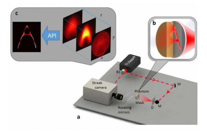
An illustration shows the researchers' experimental setup. The data captured by the camera can be thought of as a movie — a two-dimensional image that changes over time. Credit: Massachusetts Institute of Technology
