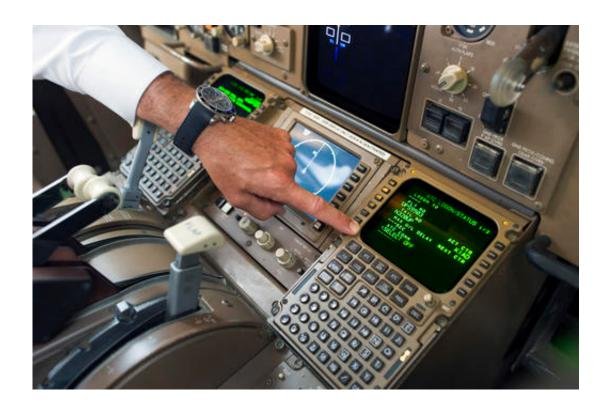
UPS Capt. Christian Kast points to the Data Communications Data Comm technology in the cockpit of an UPS Boeing 767-300F aircraft at Dulles International Airport Air Traffic Control Tower in Sterling, Va., Tuesday, Sept. 27, 2016. Data Comm gives air traffic controllers and pilots the ability to transmit flight plans, clearances, instructions, advisories, flight crew requests, and reports via a digital message service. (AP Photo/Cliff Owen)
